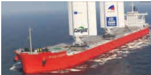
Mitsubishi Corporation's Pyxis Ocean is set to be the first vessel fitted with B&W Technologies' wind propulsion technology WindWings.
