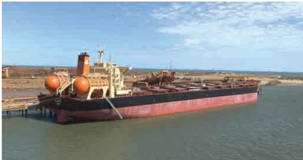
Bulk - carrier cu sistem de propulsie tip dual fuel LNG- MGO
