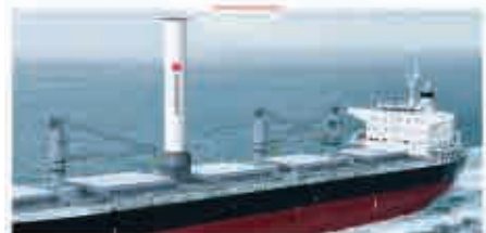
Shipping giant BHP has partnered with Pan Pacific Copper and Nippon Marine to outfit a rotor sail system aboard a geared bulkier to reduce emissions.
